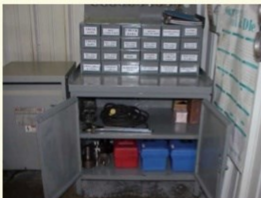
After 5S - Cleaned, organized and drawers labeled (less time and frustration hunting)
